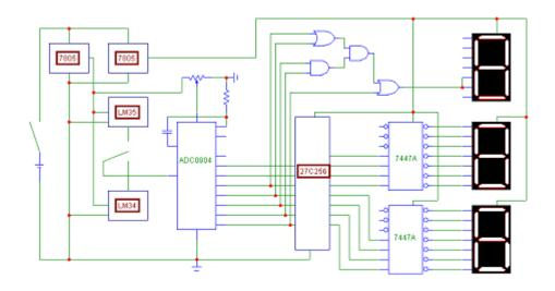
Minimum Input Voltage: 7V Sample Resolution: 0.5 Degree Display Resolution: 1 Degree Typical Current: 50mA to 100mA
